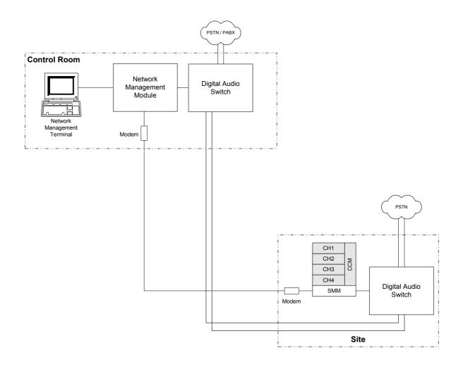
Figure 1: Where the CCM fits in a TaitNet system
