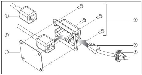
3 Slide the extension cable socket O into the housing unit.
