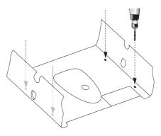
Use two screws per rail and tighten the screws to a minimum torque of 20lbf in (2.26Nm).
