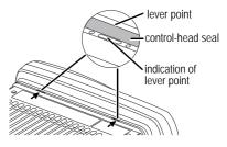
2 Use the screwdriver to lift the control head off
