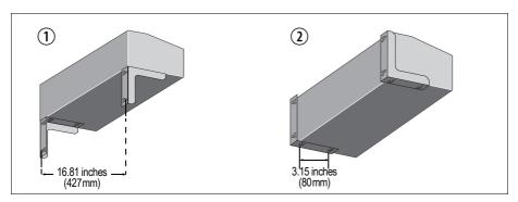
The following diagram shows the spacing of the mounting holes.
