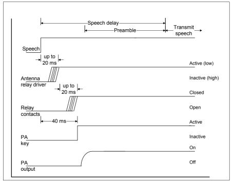
When the voter begins providing output for transmitting, the base station waits for 20ms before activating the antenna relay line (Pin 1). It then waits a further 20ms for the antenna relay to close before activating the PA key signal, which instructs the PA to begin transmitting. In digital P25 mode, it transmits the full preamble before beginning to transmit speech (speech transmission only begins after the antenna relay delay and the preamble time).
