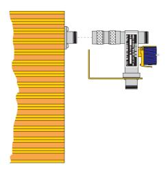
3. Secure the antenna relay bracket by fitting the supplied M3 x 8 mm screw through the bracket to the PA chassis.
