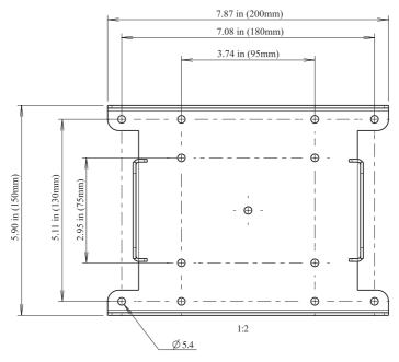
The four outer mounting holes allow for the radios to remain mounted to the cradle when mounting or fixing the cradle.
