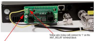
Black wire (negative from supply) connects to '2' on the 'ANT\_RELAY' terminal block
