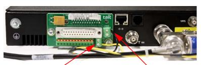
Black wire (negative from supply) connects to '-' on the 'pwr' terminal block
